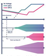
Dc voltage and AC current behaviour usin different value for delay time
